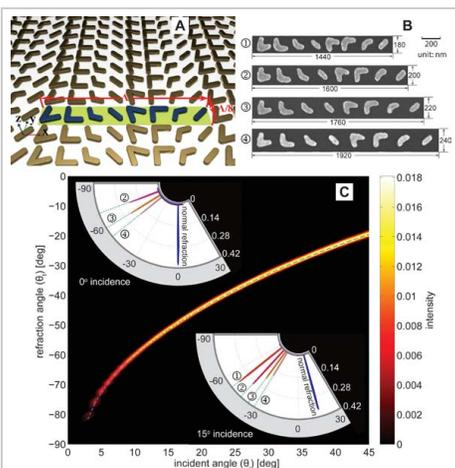
The image in the upper left shows a schematic for an array of gold "plasmonic nanoantennas" able to precisely manipulate light in new ways, a technology that could make possible a range of optical innovations such as more powerful microscopes, telecommunications and computers. At upper right is a scanning electron microscope image of the structures. The figure below shows the experimentally measured refraction angle versus incidence
