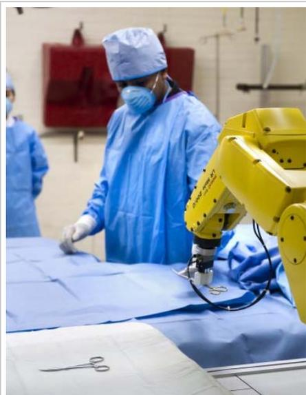
Purdue industrial engineering graduate student Mithun Jacob uses a prototype robotic scrub nurse with graduate student Yu-Ting Li. Researchers are developing a system that recognizes hand gestures to control the robot or tell a computer to display medical images of the patient during an operation. (Purdue University photo/Mark Simons)
