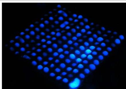
Researchers have invented a technique that uses inexpensive paper to make "microfluidic" devices for rapid medical diagnostics and chemical analysis. To demonstrate the new concept, the researchers created paper strips containing arrays of dots dipped in luminol, a chemical that turns fluorescent blue when exposed to blood. Blood was then sprayed on the strips, showing the presence of hemoglobin. (Birck Nanotechnology Center, Purdue University)
