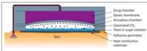
This diagram shows a new type of miniature pump activated by body heat that could be used in drug-delivery patches powered by fermentation. The micropump works by harnessing the pressure generated by fermenting yeast. Such drug-delivery patches might use arrays of "microneedles" to deliver a wider range of medications than now possible with conventional patches. (Purdue University image/Manuel Ochoa)
