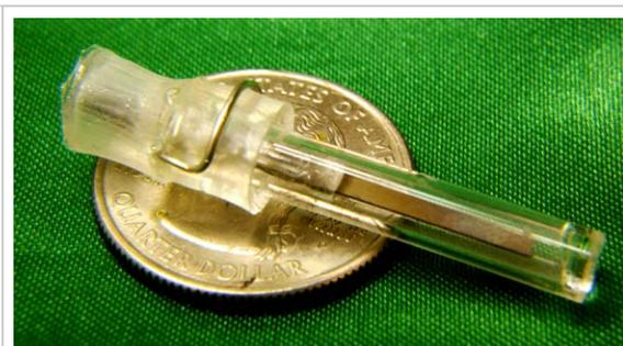
Researchers have created a new type of miniature pressure sensor, shown here, designed to be implanted in the body. Acoustic waves from music or plain tones drive a vibrating device called a cantilever, generating a charge to power the sensor. (Birck Nanotechnology Center, Purdue University)
